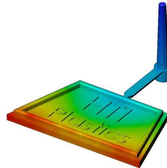
Melt temperature has a significant influence on the behavior of the polymer and the final properties of the material regardless of part design. Melt temperature is the actual temperature of the polymer as it exits the nozzle and enters the mold. The barrel set points represent the tools we use to arrive at the desired melt temperature, but they are not the same thing.
